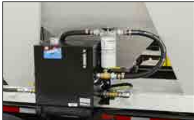
Fig 47 - Hydraulic oil reservoir
