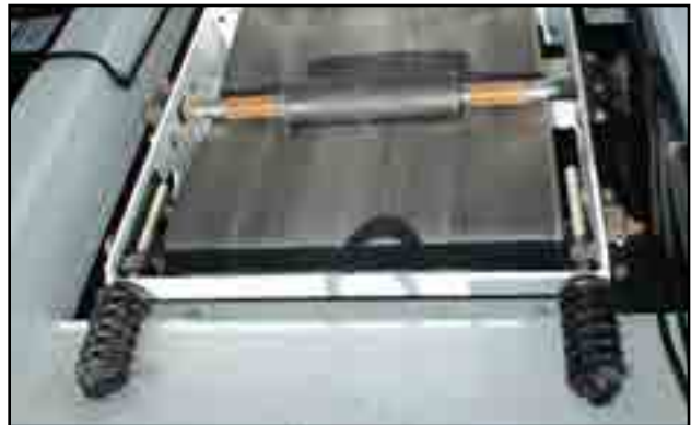
Fig 52 - Tension bolts, slave conveyor
