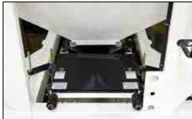
Fig 61 - Tension bolt on slave conveyor
