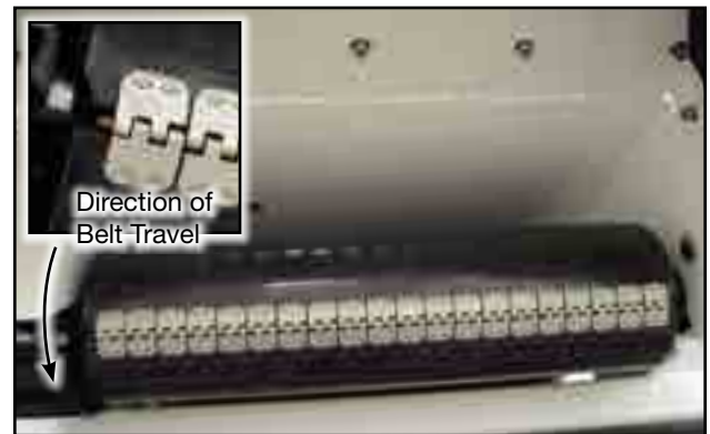
Fig 63 - Slave conveyor belt lacing
