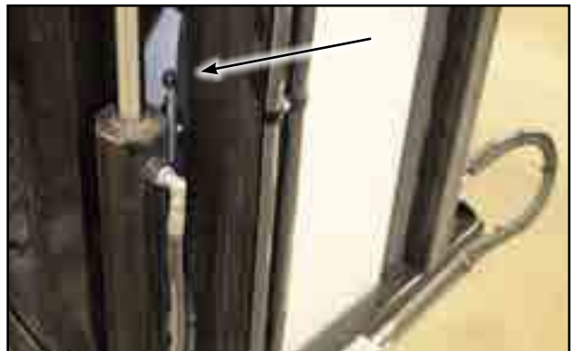
Fig 53 - Tension bolts on rear, fold conveyor
