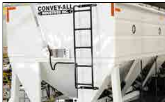
Fig 22 - Front exterior ladder
