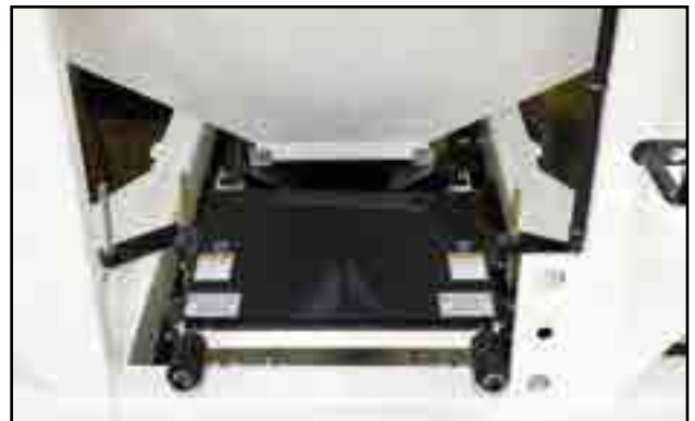
Fig 59 - Slave conveyor tension bolt and springs
