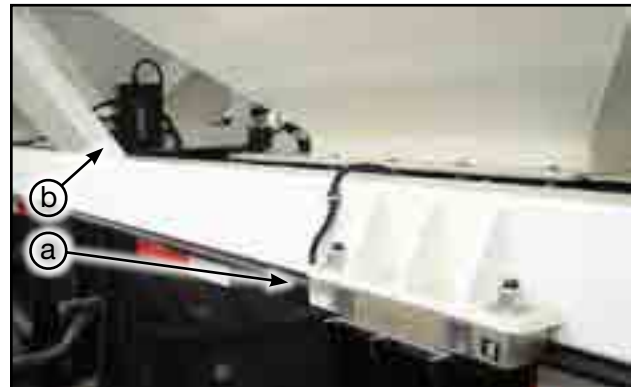
Fig 24 - (a) Load Cell, (b) weigh scale junction box
