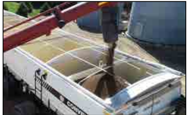
Fig 32 - Filling the hopper
